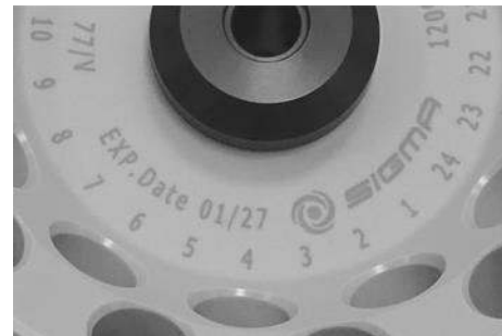
Fig. 4: Different service life – engraving on the bucket/rotor
