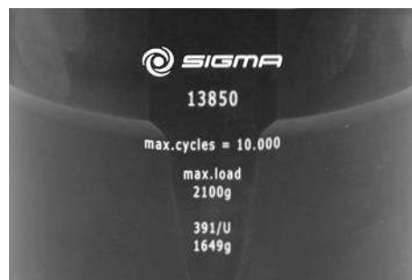
Fig. 4: Different service life – engraving on the bucket/rotor
