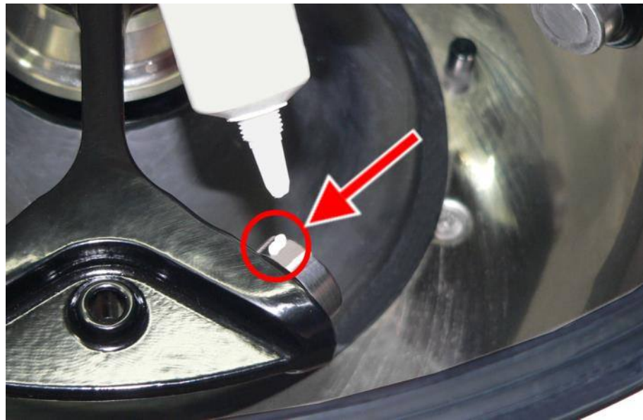
Fig. 34: Sufficient quantity of grease for one bolt
