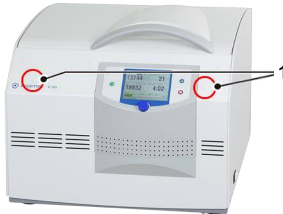
Fig. 32: Position of the openings for the emergency lid release
