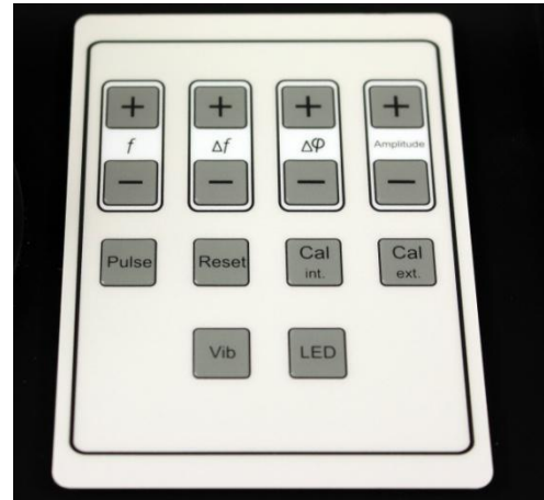
Fig. 3: The 14 keys control panel is situated on the top of the housing of the ripple tank.
