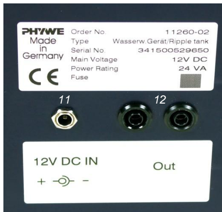
Fig. 4: Socket for the power supply (11) and sockets for the connection of the external vibration generator (12).
