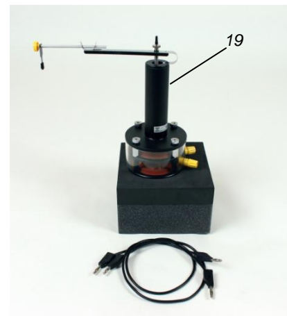
Fig. 6: External vibration generator (11260-10) with accessories, separately available.
