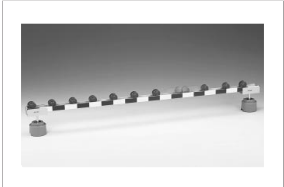
Fig. 1: Magnetic Rollers Apparatus set up for an experiment demonstrating „longitudinal waves“.
