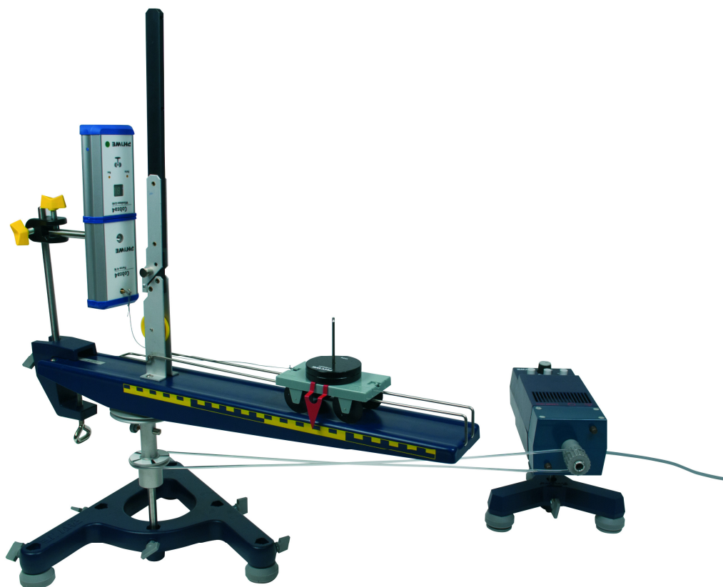
Fig. 2 Dependence of the centrifugal force on the radius of the orbit and the mass, measured with Cobra4.
