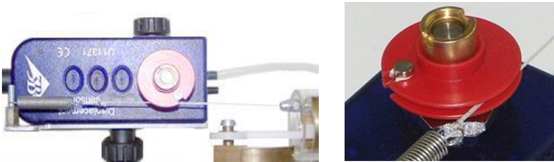
Fig. 2 Attachment of the thread to displacement sensor pulley
