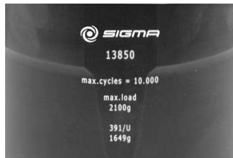
Fig. 4: Different service life – engraving on the bucket/rotor
