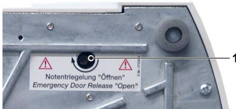
Fig. :10 Opening for the emergency lid release at the bottom of the centrifuge
