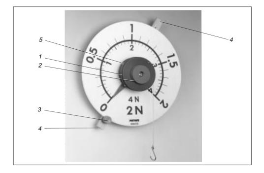
The torsion force meter is used to measure forces when carrying out experiments with the demonstration board for physics (order no. 02150.00). It has two measurement ranges, 2 N and 4 N.
