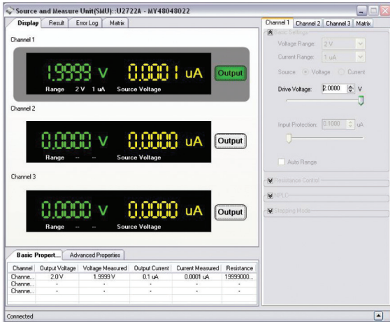
Configure all three channels separately to source or measure voltage or current.
