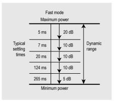
Figure 8. Auto-filter, default resolution, 10 dB decreasing power step
