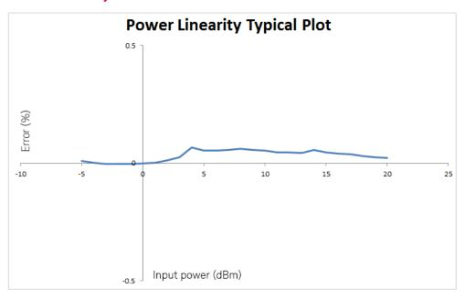
Figure 1. Typical U8480 Series power linearity at 25  $^{\circ}$ C with measurement uncertainty of  $\pm$  0.21%
