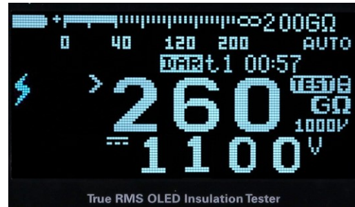
Adjustable insulation test voltage up to 1.1 kV
