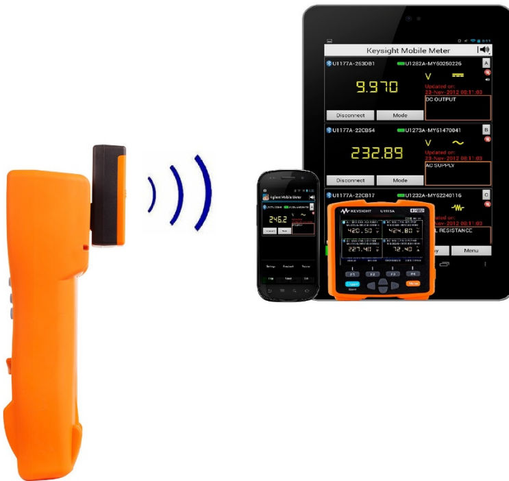
Figure 7. Pair up the U1280 series with Keysight Remote Link solution for wireless measurement option
