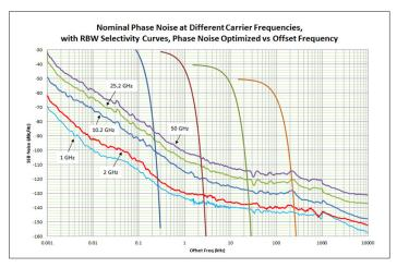
Figure 4. Nominal PXA phase noise at various center frequencies with DDS LO (Option EP0).
