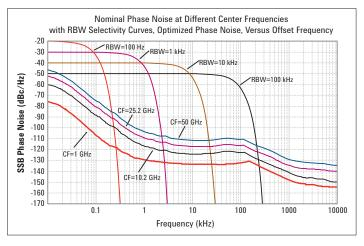
Figure 3. Nominal PXA phase noise at various center frequencies with standard LO.  $\ensuremath{\mathsf{LO}}$
