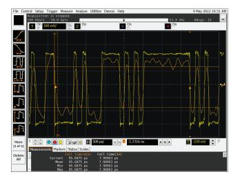
8.2Gbps PRBS^7 signal measured on Keysight 90000 Q-Series oscilloscope. Orange is the original signal with 95ps rise time. Yellow is the signal after being buffered by the N2806A. Notice the measured sub-8ps rise time and elimination of ISI.
