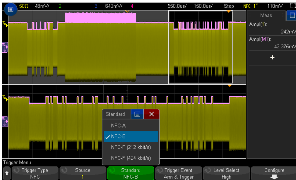
Figure 3. Using the scope's NFC trigger mode to manually characterize the Poller NFC-B modulation depth after automated test failure on the production line.
