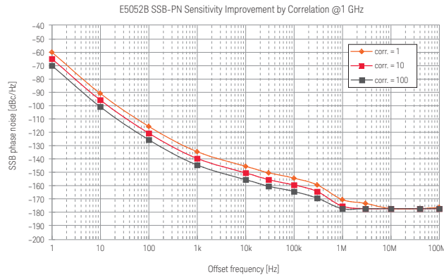
Figure 1-3. SSB phase noise sensitivity improvement by correlation (E5052B, SPD) (carrier 1 GHz, LO < 150 kHz optimized, +5 dBm input, start offset frequency = 1 Hz)
