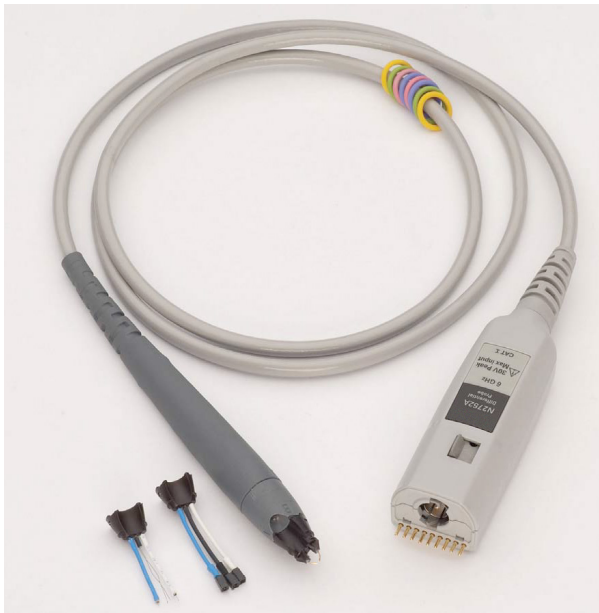
Figure 3. Keysight's InfiniiMode N2750A Series differential active probe.
