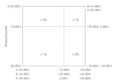
Figure 2. Relative mode power measurement linearity with an EPM Series power meter, at  $25~^{\circ}\text{C} \pm 10~^{\circ}\text{C}$  (typical).
