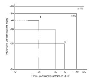
Figure 1. Relative mode power measurement linearity with EPM Series power meter/E-Series CW power sensor at 25  $^{\circ}$ C  $\pm$  5  $^{\circ}$ C (typical).
