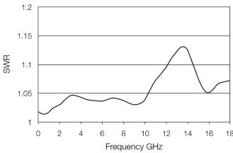
Typical SWR, 10 MHz to 18 GHz (25  $^{\circ}$ C  $\pm$  10  $^{\circ}$ C) for E9300H and E9301H sensors.
