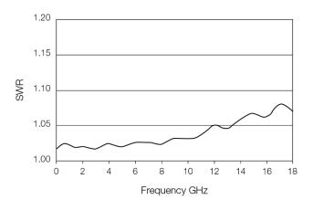
Typical SWR, 10 MHz to 18 GHz (25  $^{\circ}$ C  $\pm$  10  $^{\circ}$ C) for E9300B and E9301B sensors.
