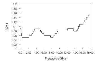
Typical SWR, 10 MHz to 18 GHz (25  $^{\circ}$ C  $\pm$  10  $^{\circ}$ C) for E9300A and E9301A sensor.
