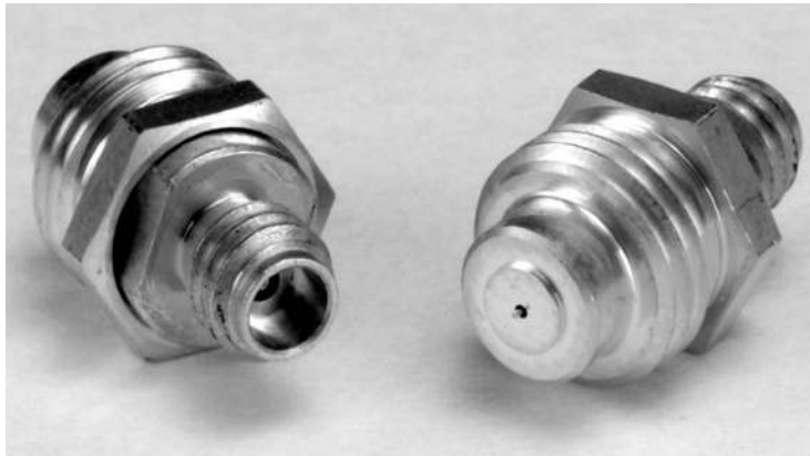
A pair of 1.0 mm female connector launch assemblies. Left: 1.0 mm female connector end Right: Package end with 0.162 mm diameter pin
