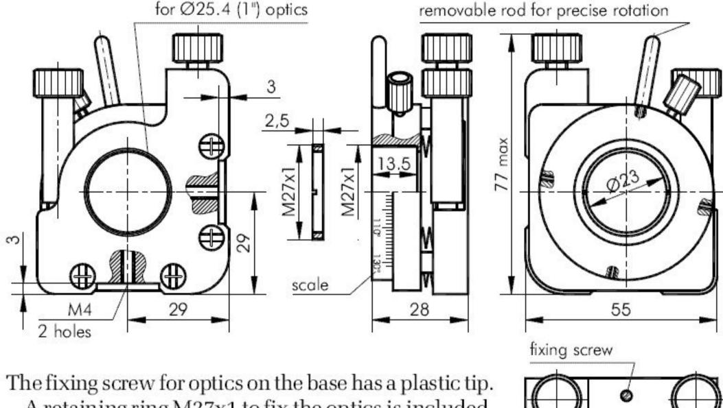
The fixing screw for optics on the base has a plastic tip. A retaining ring M27x1 to fix the optics is included. A tightening key **3K-25** for the retaining ring is available on request.
