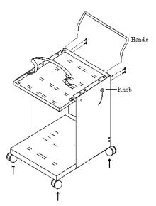
The knob on each side is used to lock the position of the tilt tray. However, these knobs are not installed in the unit as shipped (to protect the knobs from damage). Instead, packing screws lock the tray for shipment. Remove the packing screws (discard) on each side and replace it with the knob provided. Tighten the knobs to lock the tray.
