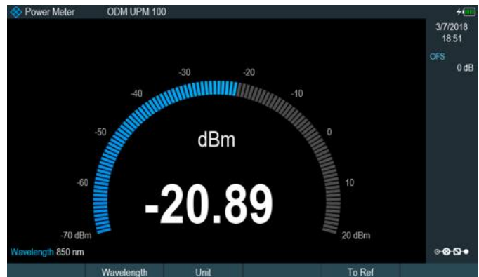
Optical power measurement with optical power sensor.
