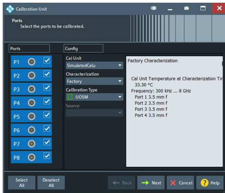
Figure 6-11: Calibration Unit wizard, step 1: Ports (> 4 test ports)
