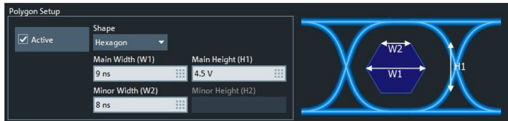
Figure 6-67: Center polygon setup: hexagon
