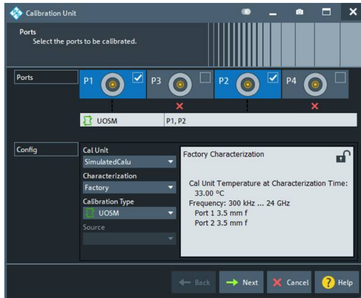
Figure 6-10: Calibration Unit wizard, step 1: Ports
