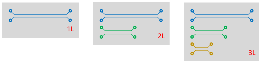
Figure 5-24: Test coupons for 1L, 2L and 3L measurements
