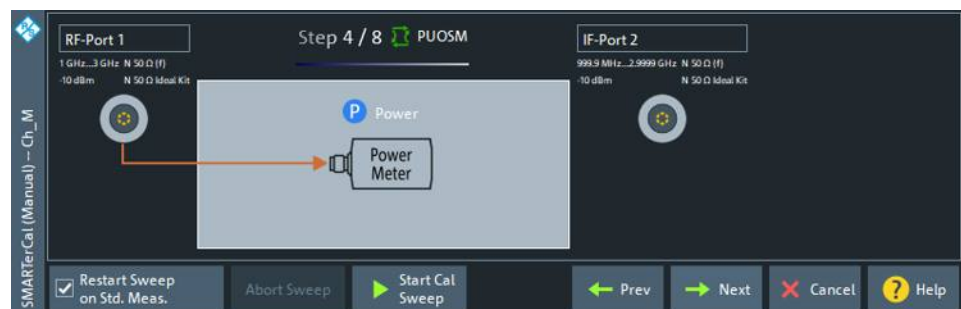
Figure 6-45: Scalar Power Calibration
