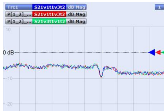
Figure 6-14: Multiple traces due to multiple paths
