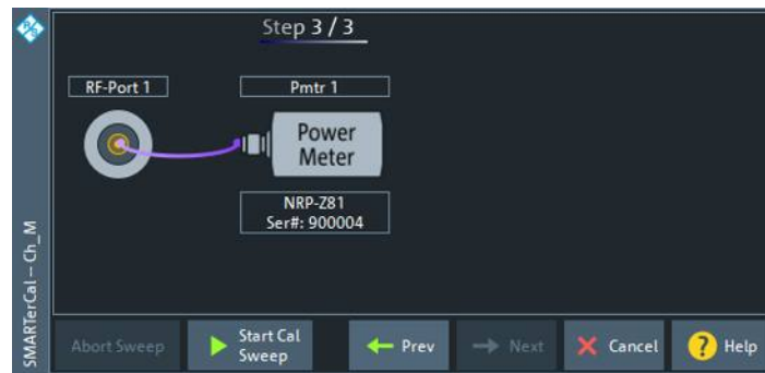
Figure 6-43: Scalar Power Calibration
