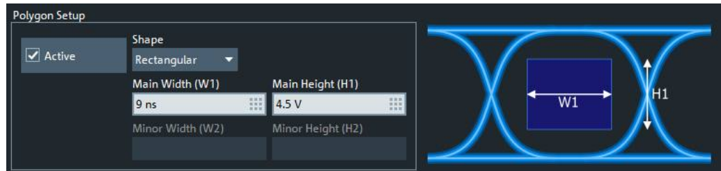
Figure 6-68: Center polygon setup: rectangle
