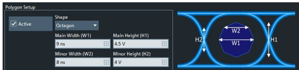
Figure 6-66: Center polygon setup: octagon
