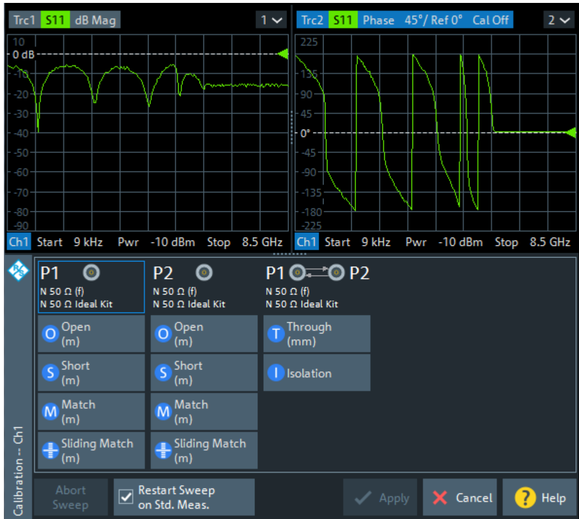
Figure 6-20: Calibration Setting Wizard, Step 3: Calibration
