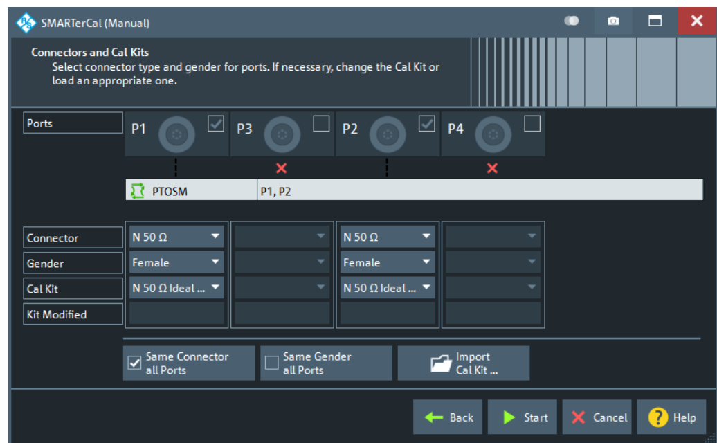
Figure 6-31: SMARTerCal(Manual), Step 2: Connectors and Cal Kits
