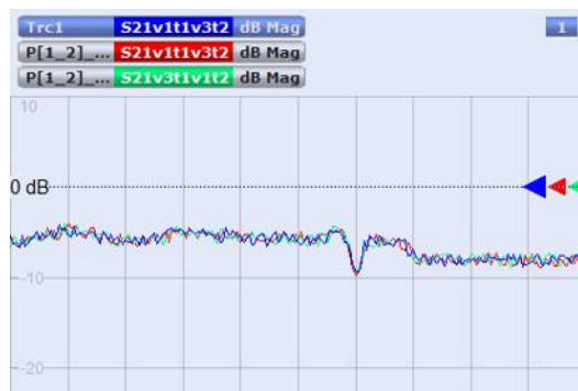
Figure 6-33: Multiple traces due to multiple paths
