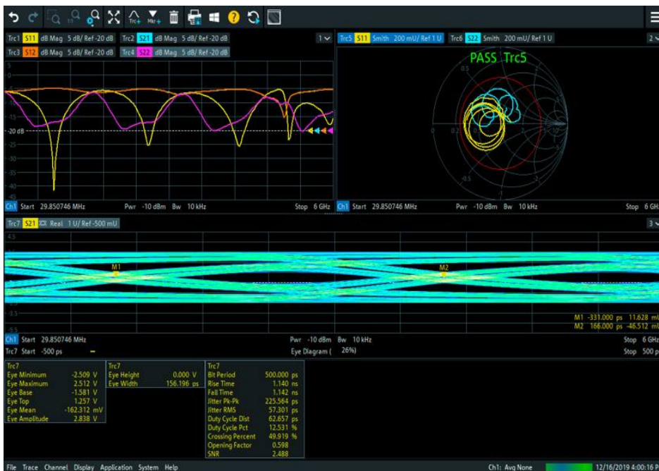
Simultaneous display of eye diagrams and measurements in the frequency and time domain.
