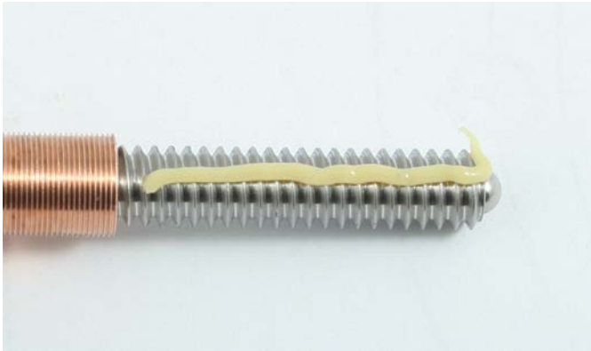
Fig. 4.1 Greasing the Leadscrew
