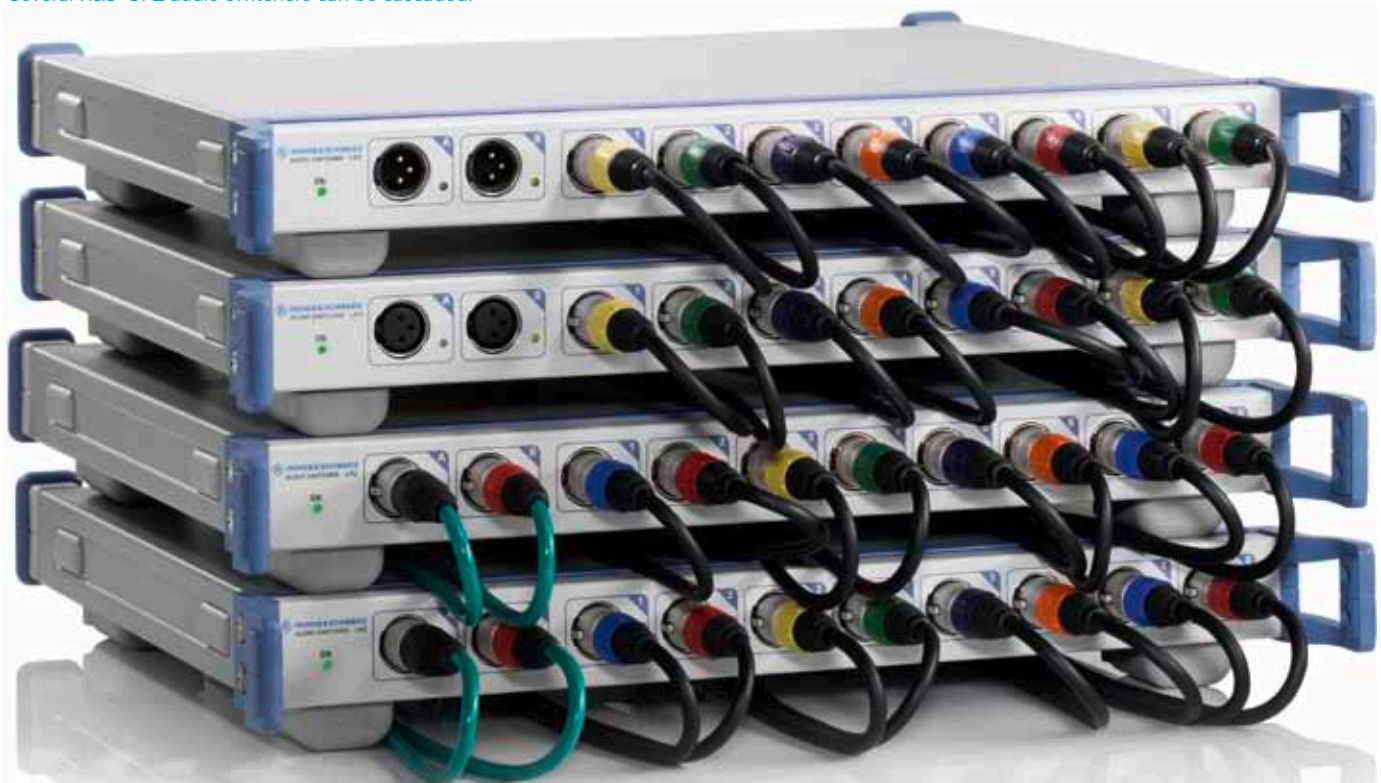
Several R&S®UPZ audio switchers can be cascaded.
