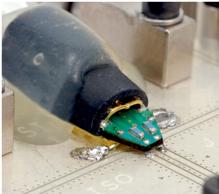
Figure 16: Typical wire length from probe tip to circuit
