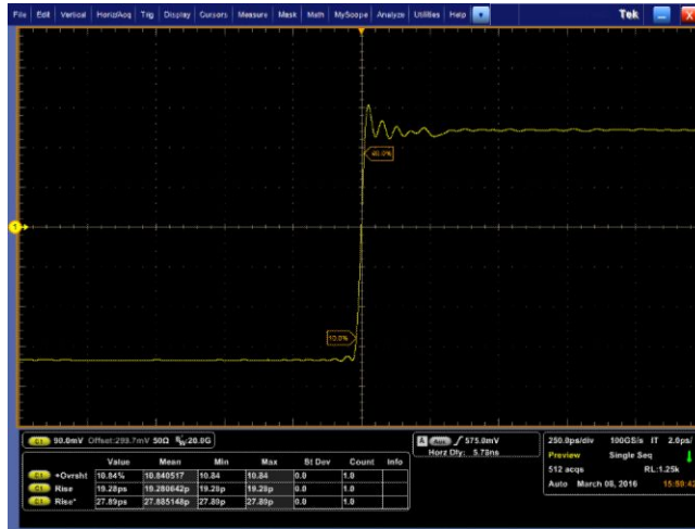
Figure 17: P77STFLXA solder tip attached with 75 mils (1.90 mm) wires (rise time = 27.9 ps)
