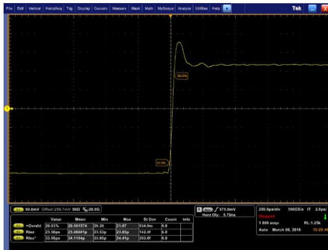
Figure 19: P77STFLXA solder tip attached with 200 mils (5.08 mm) wires (rise time = 34 ps)
