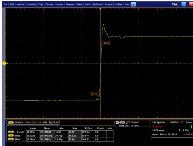
Figure 18: P77STFLXA solder tip attached with 120 mils (3.05 mm) wires (rise time = 30.1 ps)
