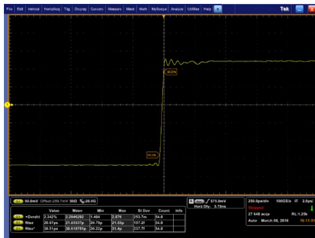
Figure 16: P77STFLXA solder tip attached with 10 mils (0.250 mm) wires (rise time = 30.5 ps)
