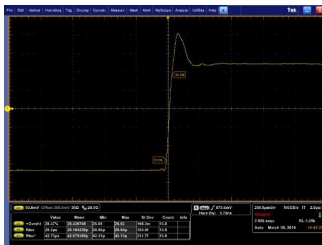
Figure 20: P77STFLXA solder tip attached with 300 mils (7.62 mm) wires (rise time = 42.8 ps)
