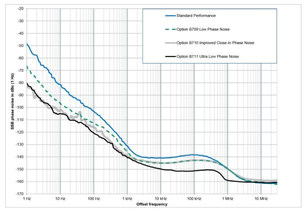
Measured SSB phase noise performance at f = 1 GHz, CW mode, standard performance versus the R&S $^{\circ}$ SMW-B709, R&S $^{\circ}$ SMW-B710 and R&S $^{\circ}$ SMW-B711 options
