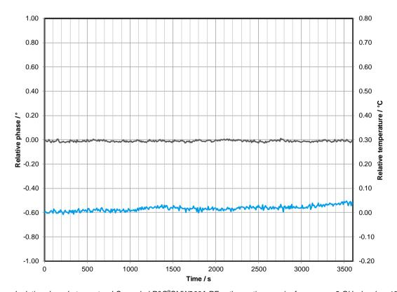
Measured relative phase between two LO coupled R&S $^{\otimes}$ SMW200A RF paths vs. time, carrier frequency = 2 GHz, level = -10 dBm (the lower curve/right vertical axis indicates the temperature variation)
