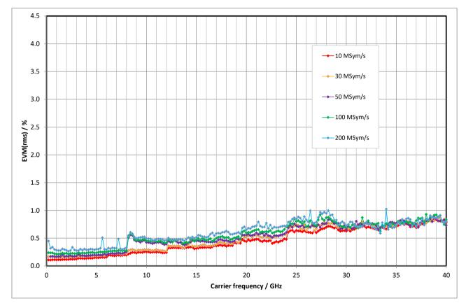
Measured EVM versus carrier frequency for 16QAM
