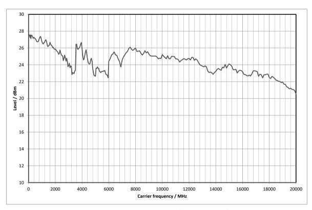
$\textit{Measured maximum available output level versus frequency with R\&S §SMW-B1020, R\&S §SMW-B2020 frequency options and the state of the$
