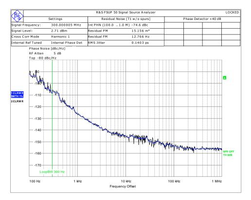
Measured phase noise of wideband analog I/Q outputs; single-ended sine wave with f = 300 MHz
