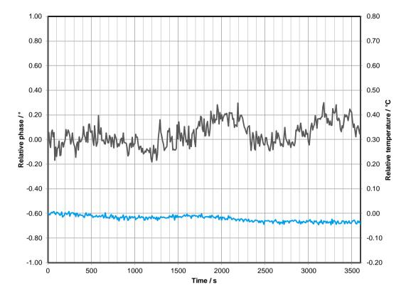
Measured relative phase between two LO coupled R&S $^{\otimes}$ SMW200A RF paths vs. time, carrier frequency = 40 GHz, level = -10 dBm (the lower curve/right vertical axis indicates the temperature variation)
