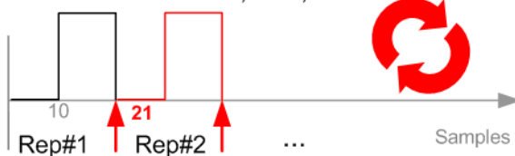
Figure 4-22: Example: Processing of MARKER TRACE if CONTROL LENGTH is not used
