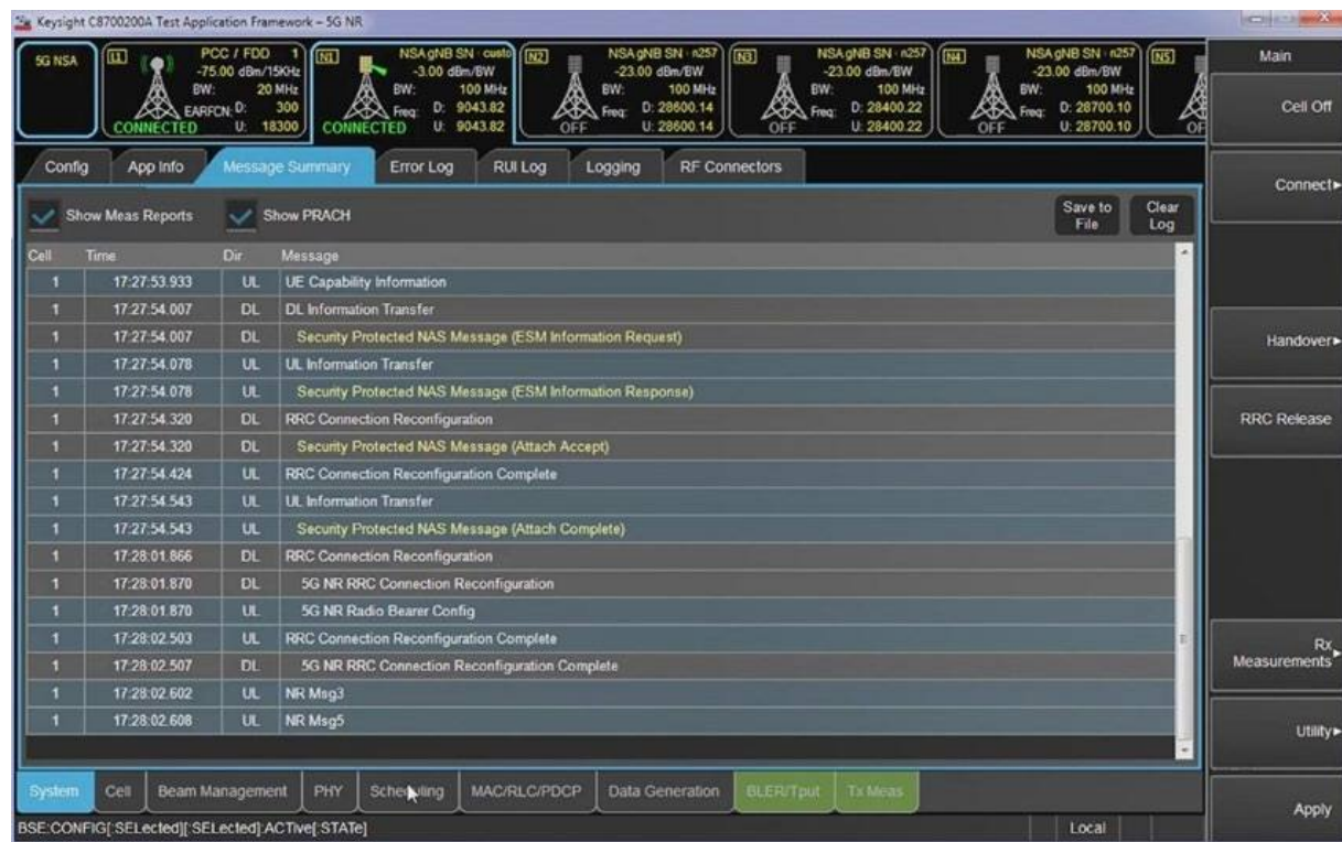
Figure 1. Screen capture illustrating a completed 5G NR NSA Random Access procedure using Keysight's 5G Test Application Framework
