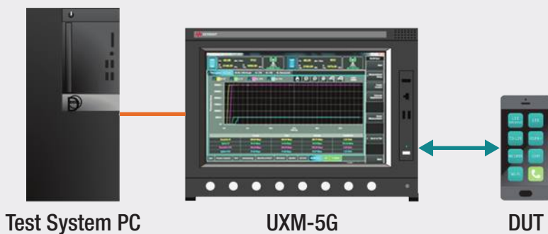
Figure 11 - Test setup for sub-6GHz in Standalone or Non-Standalone mode.
