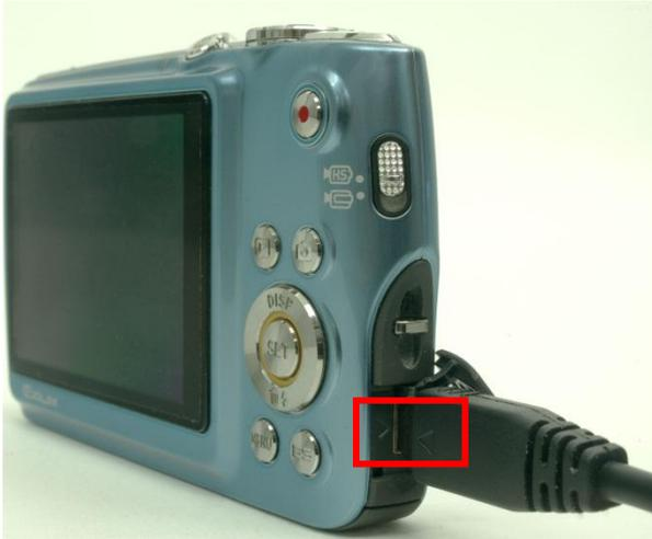
**Image 8:** How to connect the camera to a computer with the USB cable provided.
