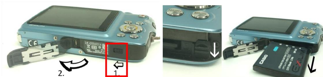
**Image 1:** How to open the camera base and remove the battery.
