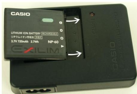
**Image 2:** How to insert the battery in the charger provided.
