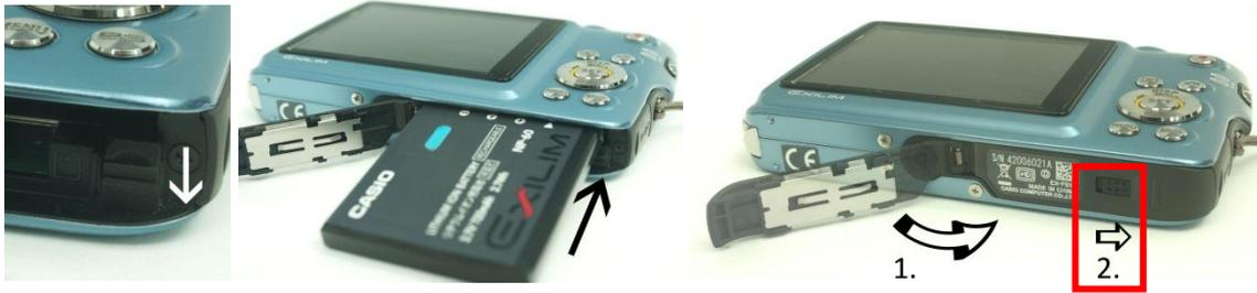
**Image 3:** Correct insertion of camera battery, closing the camera base cover.
