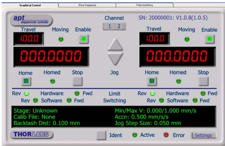
Fig. 5.3 Motor controller software GUI (dual channel version)
