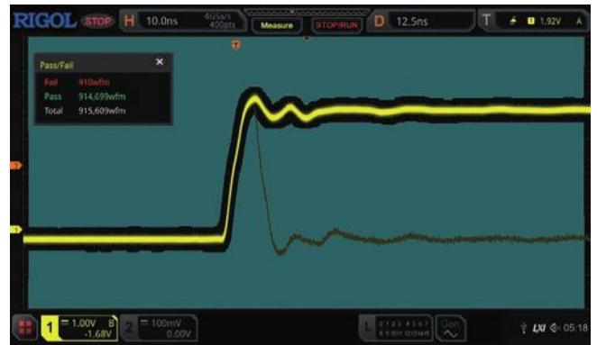
The Pass/Fail test function can quickly make a statistics on the occurrence probability of the signal exceptions.
