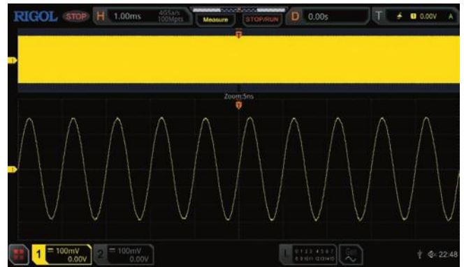
With up to 100 M memory depth, you can capture 12.5 ms of waveforms while maintaining a sample rate of 4 G, without causing the waveforms to be distorted.
