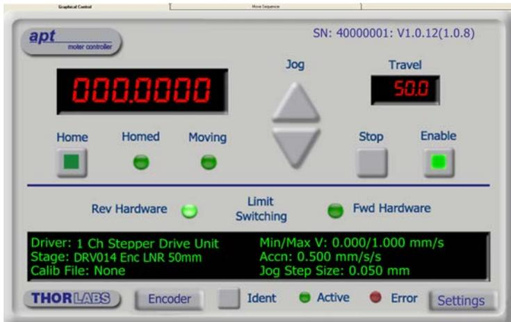
Fig. 7.2 Motor GUI panel with encoder button
