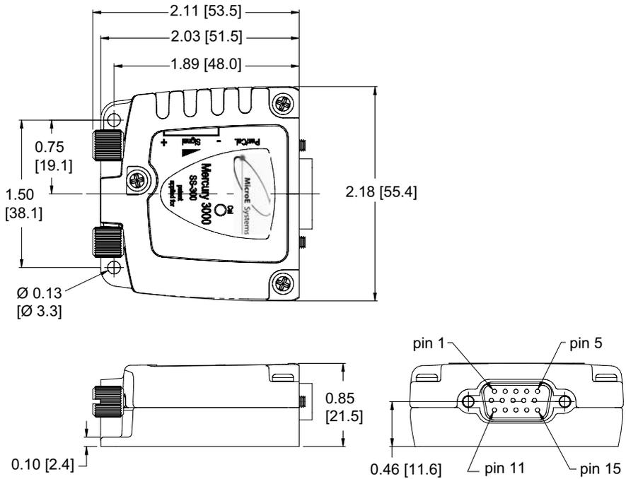
Fig. 5.2 Dimensions – SmartSignal electronics module
