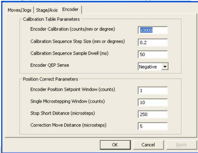
Fig. 7.4 Motor settings - Encoder tab
