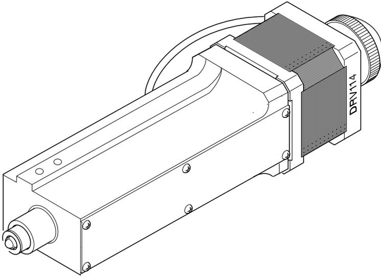
**Fig. 1.3 A typical stepper motor drive**
