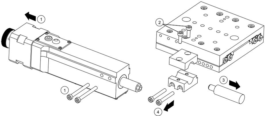
**Fig. 3.7 Removing the Actuator Clamp and Push Block**
