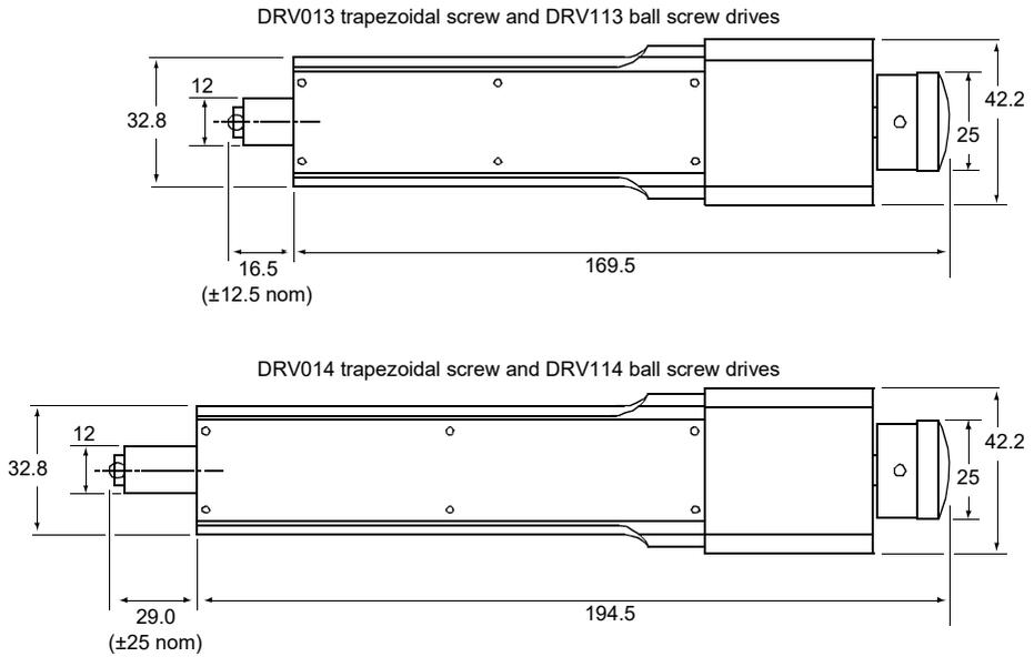
**Fig. 5.3 Dimensions – stepper motor drives**
