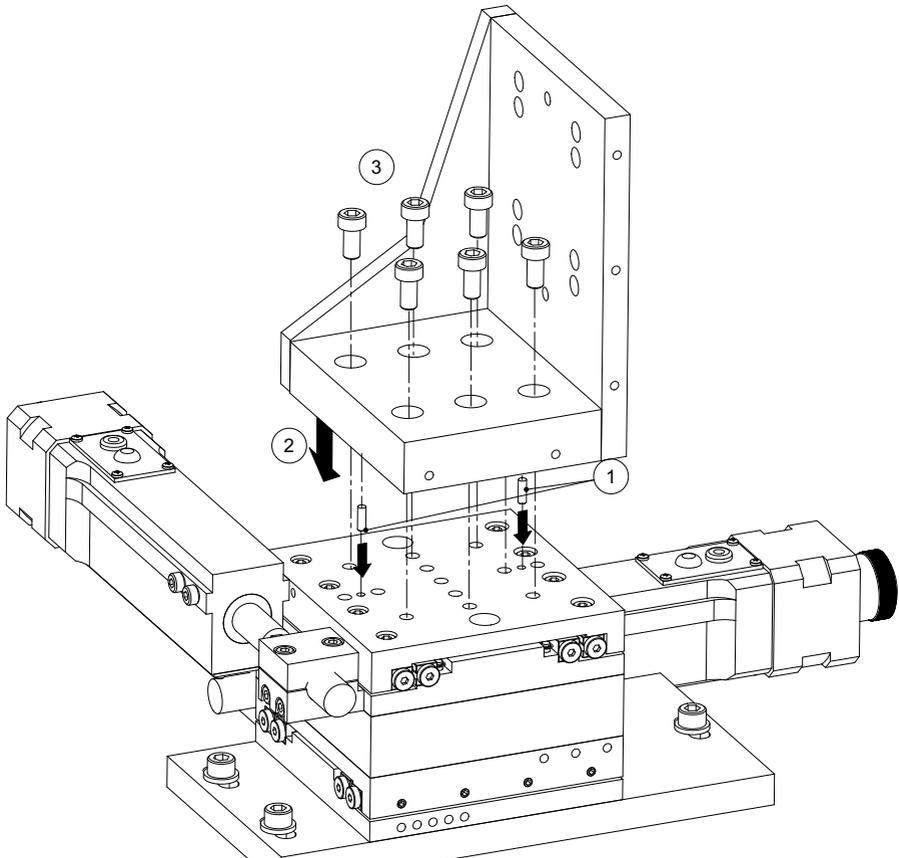
**Fig. 3.4 Fitting the Angle Bracket**
