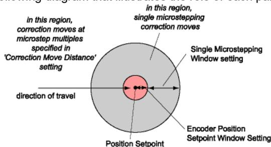
Fig. 7.5 Positioning correction mode parameters
