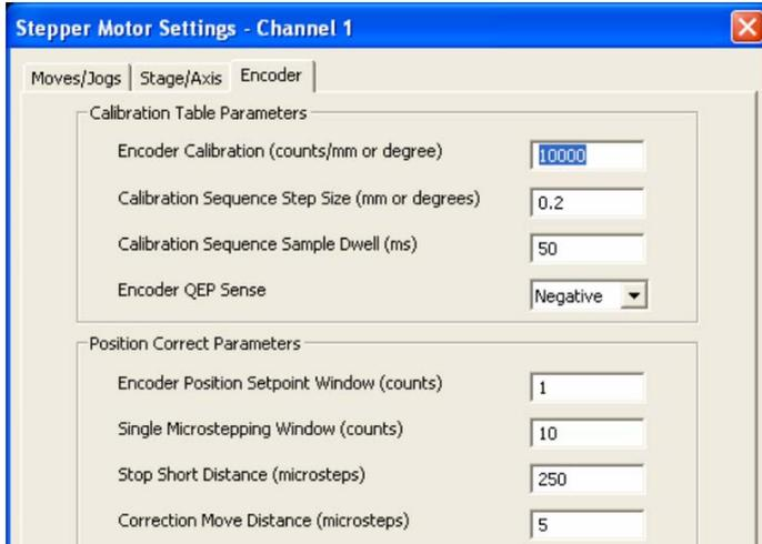
**Fig. 7.3 Motor settings - Encoder tab**
