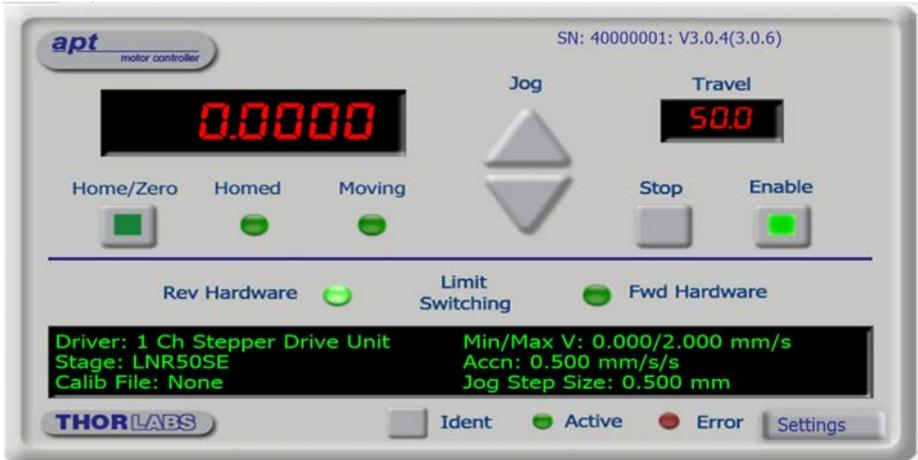
Fig. 4.7 Motor GUI panel with encoder button
