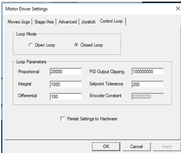
Fig. 4.8 Settings - Control Loop tab
