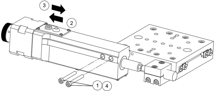
**Fig. 3.6 Fitting/removing a motor drive**
