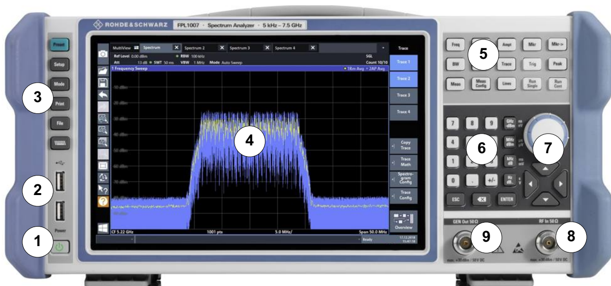
Figure 5-1: Front panel view of R&S FPL1000
