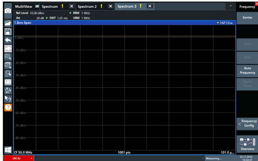
Figure 5-10: Time domain display of the calibration signal
