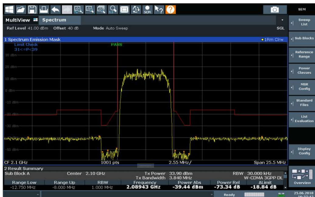
Figure 7-26: Detected peak display in SEM measurement
