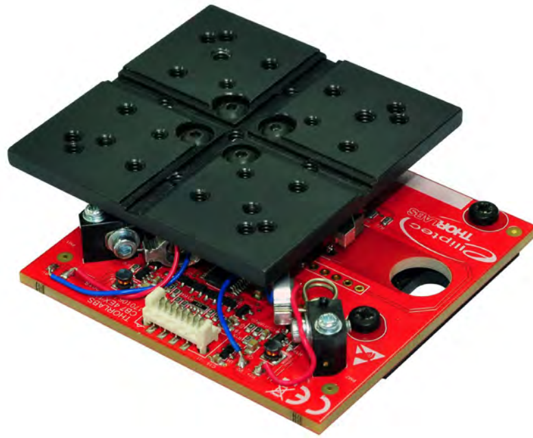
Figure 2 ELL17 with MMP1 Top Plate Fitted, Showing Stage in Backwards/Home Position
