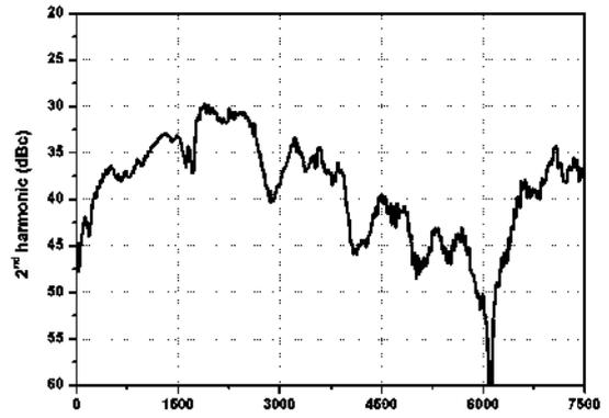
Measured tracking generator output 2<sup>nd</sup> harmonic of DSA832/DSA875
