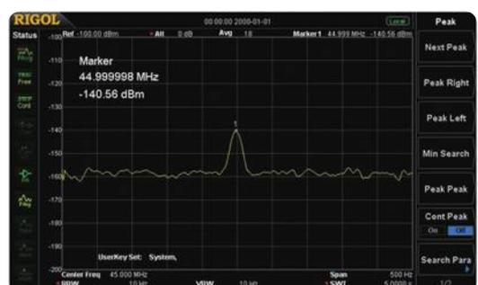
Phase noise < -98 dBc/Hz @10 kHz offset (DSA832/875/832E)
