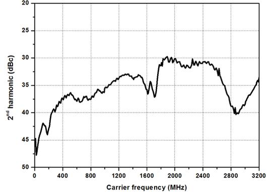
Measured tracking generator output 2<sup>nd</sup> harmonic of DSA832E
