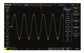
Built-in dual-channel 25 MHz source (DS1XX4Z-S Plus)
