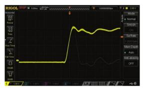
UltraVision: waveform recording and playback functions
