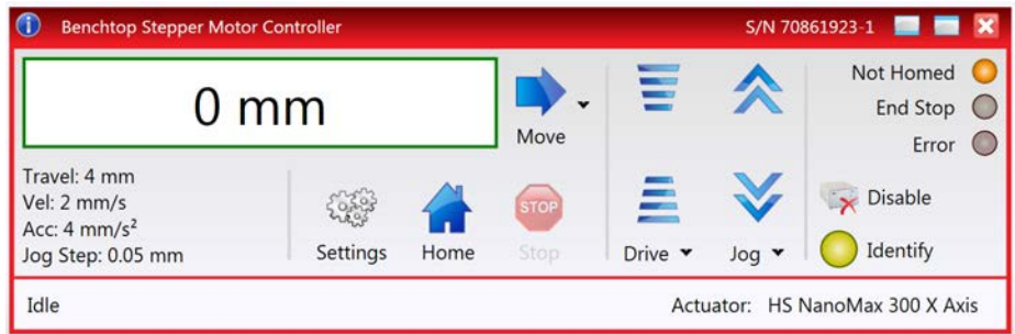
Fig. 3.4 Gui panel showing jog and ident buttons
