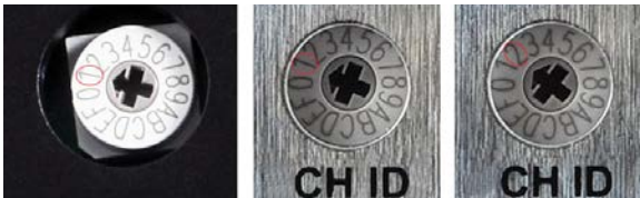
Fig. 4.1 ID switch settings
