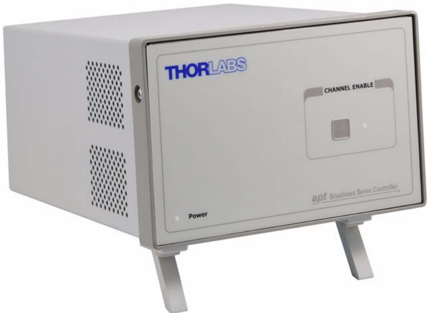
Fig. 2.1 APT Single Channel Brushless DC Servo Motor Controller (BBD201)
