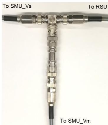
Figure 2-6. Triax TEE configuration using adapters.
