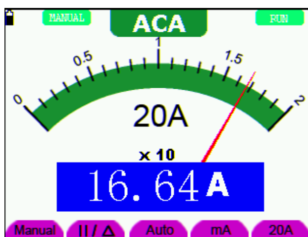
figure 27: AC Current Measurement for 20A
