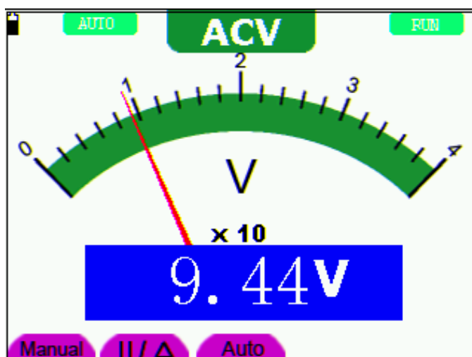
figure 23: AC Voltage Measurement
