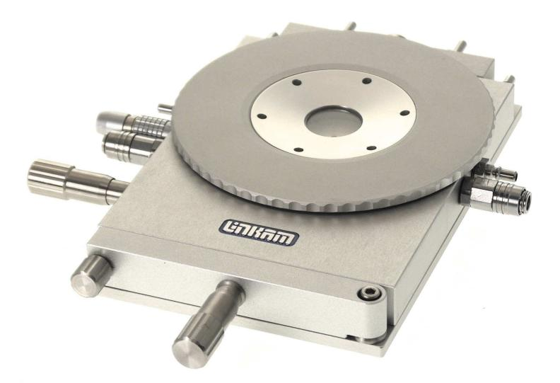
**Heating and Freezing** Temperature range from –196°C up to 600°C **Optical Techniques** Light Microscopy, Raman, X-ray, Confocal and more **Rapid and Slow Heating** Wide range of heating rates from 150°C/min to 0.01°C/min
