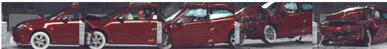
Crashtest, single extracted images of sequence - original resolution 2016 x 2016 @ 1102 frames/s (color version)
