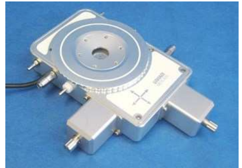
The MDS600 heating and freezing stage
