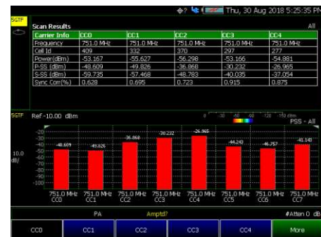
5G TF OTA measures control channels and displays cell ID
