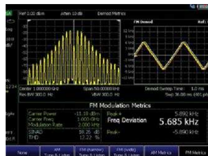
Characterize AM/FM signals using AM/FM demodulation
