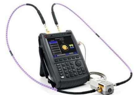
Perform fast and accurate calibrations using ECal
