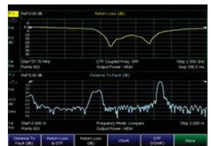
View return loss and DTF simultaneously
