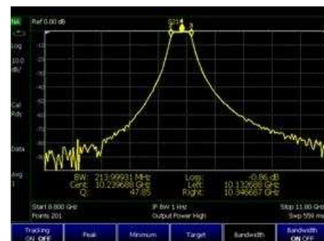
Use the marker bandwidth/Q factor function to simplify filter testing and tuning
