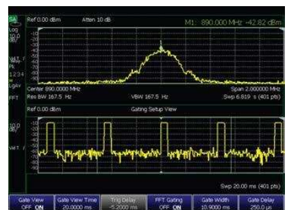
Analyze pulsed RF signals using the time-gating option
