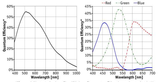
${}^{\star}\text{QE measured without protection glass or filters. With glass or filters, quantum efficiency decreases by approximately 10\%.}$
